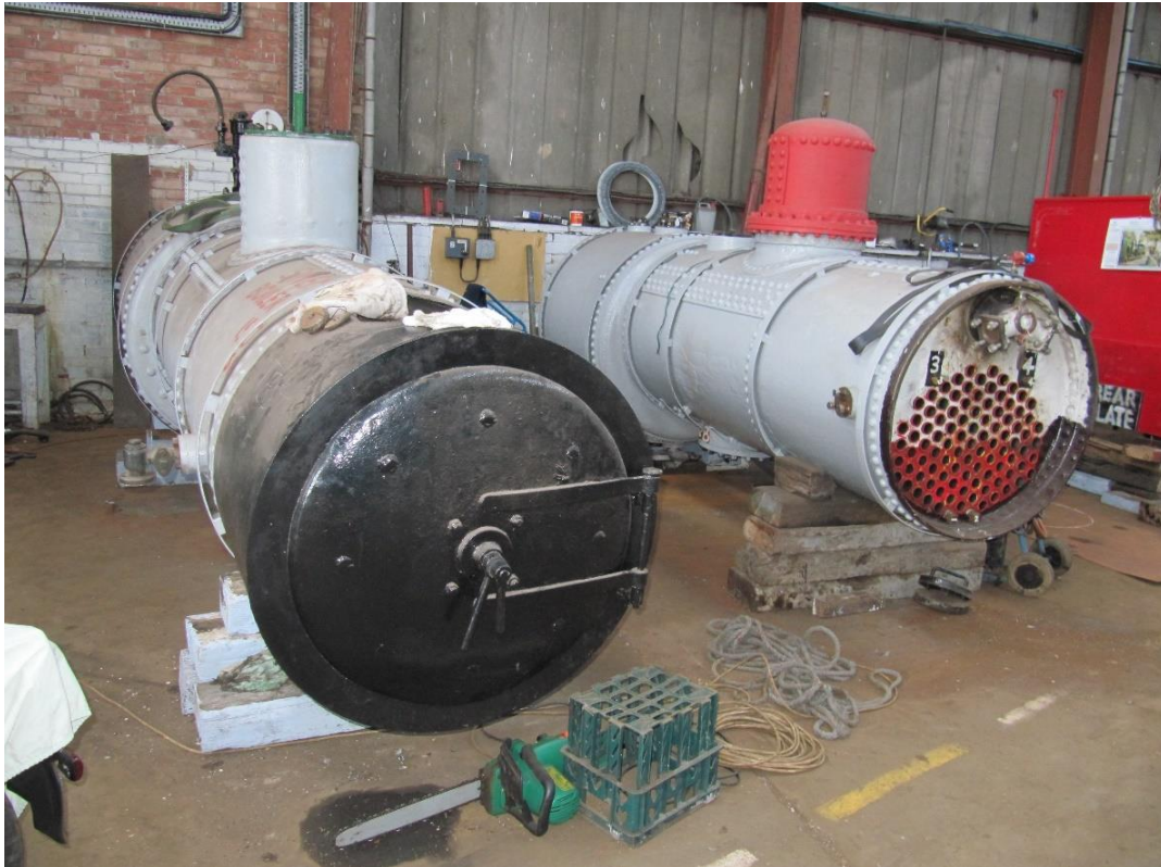
Boilers of 'SINEMBE' (left) and 'A BOULLE' (right) without its smokebox at Riverside in September 2010
