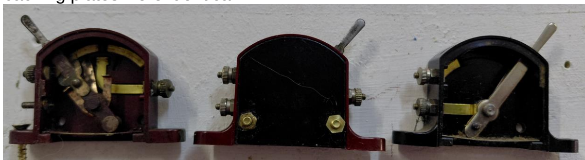
Point switch without backing plate left and with backing plate middle. Simple (on/off) isolating rail switch without backing plate right. Note three terminals for point switches and only two for isolating rails.
