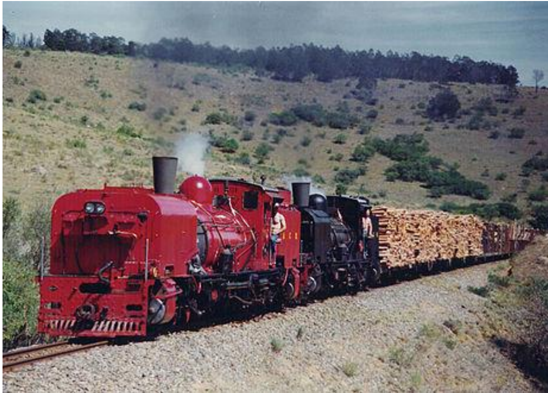
The two NGG16A locos climbing the hill to Nquabeni c1992. Both locos now reside in operational condition at Sandstone Estates. Photo Wikipedia.
