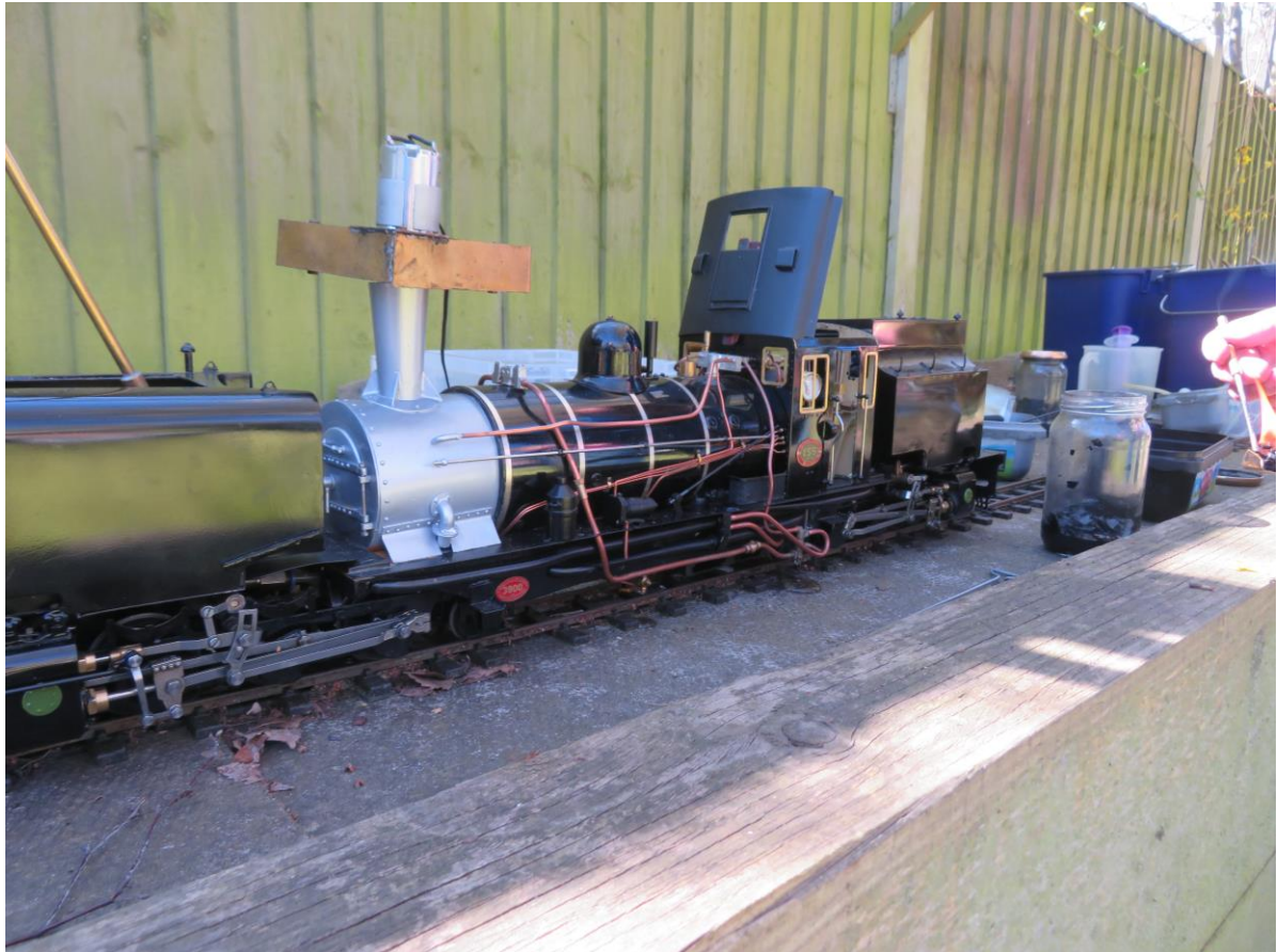
NGG16A in the steaming bay. Note lever for hand water pump in front tank and battery powered blower in chimney.
