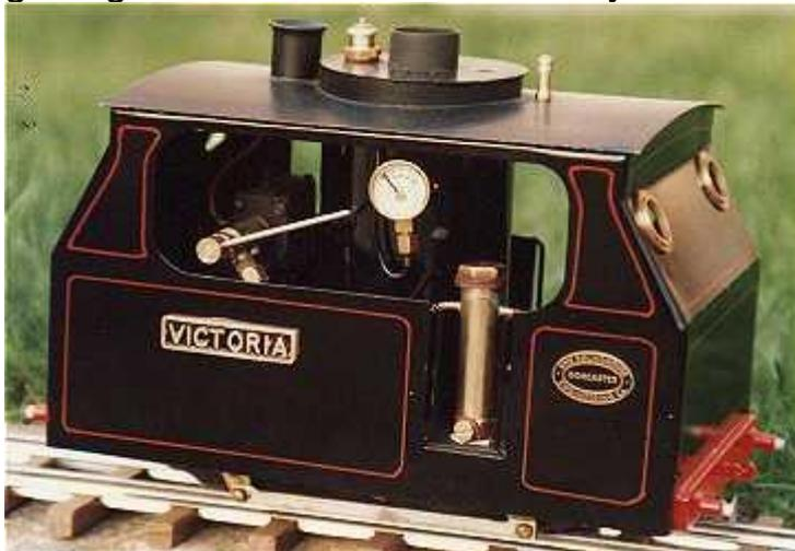
**“The first commercial model from the Roundhouse stable! 'Victoria' was a model of an 0-4-0 vertical boilered tram locomotive that ran on the Plynlimon and Haffan Railway and was launched in February 1982. She had a single cylinder operated by slip-eccentric valve gear and a spirit fired vertical boiler.”**
