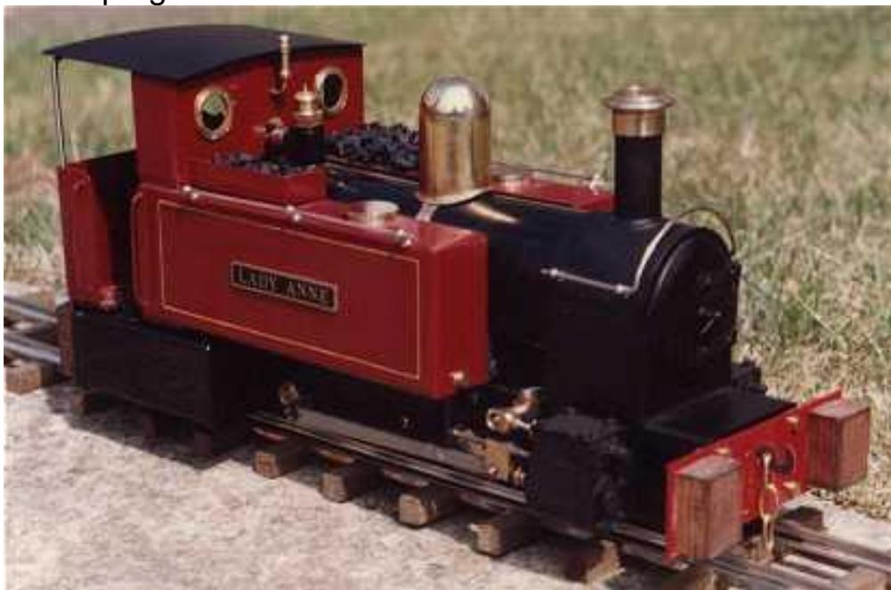
***Lady Anne Mk 2 in 1984 now with a cab. In the same year tinplate was replaced with photo etched brass platework,***
