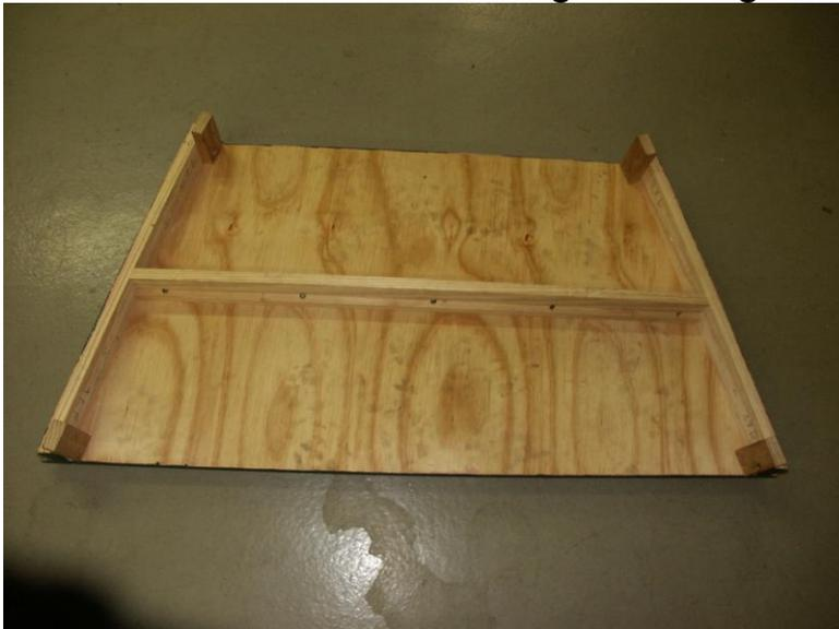
The boards were braced with 2x1 'T' beams down the centre which are secured into 3x1 end pieces running crosswise (refer photograph below of corner board)
