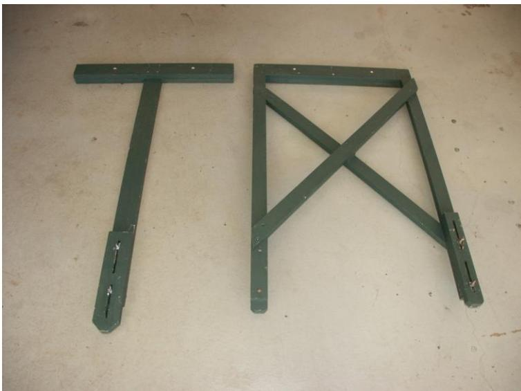
There are two types of trestles. The first, uses 2x1 pine for the legs and cross bracing with two 3x1 cross members back to back at the top. The second comprised two 3x1 cross members back to back and a single 3x1 leg.
